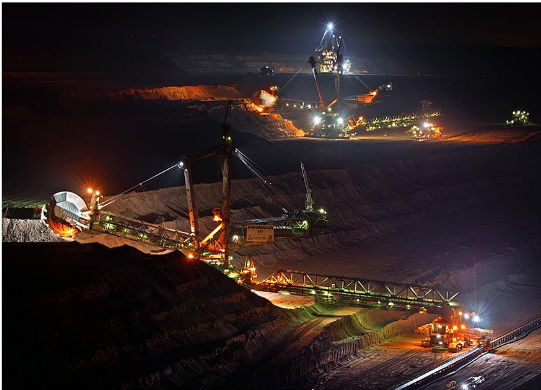
Image: use of a bucket wheel excavator for surface mining in Hambach
